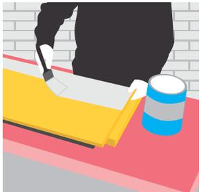
Apply a thin, uniform layer of primer by hand to the panel surfaces where the 896 PanelFIX adhesive will be applied. Samrat recommends Dow Corning Primer P.
