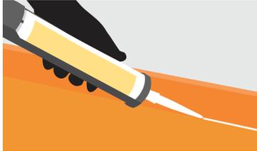
After tape installation, apply the adhesive on to the supporting structure and also directly to the panel. Apply the adhesive in a continuous operation using a caulking gun, allowing a minimum of 5mm distance from the tape, Extrude the silicon Adhesive with minimal angle between of nozzle and the surface to achieve required joint dimensions.
